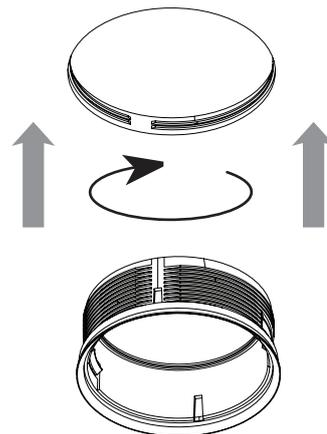
③ Use tightening tool to turn the housing so it aligns with the ceiling.
