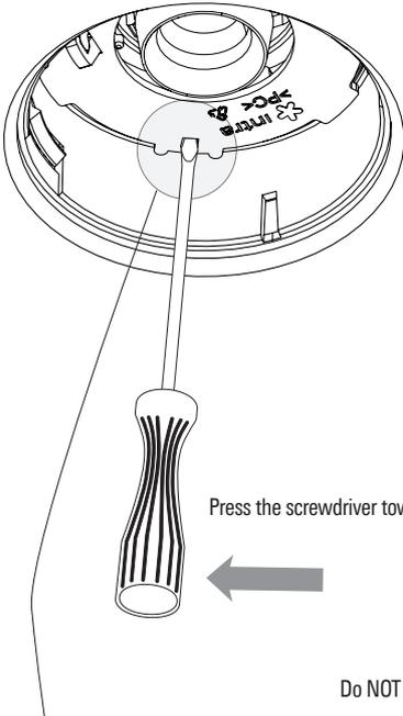
Press the screwdriver towards the housing to release the pins.
