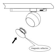
Install the magnetic reflector if not mounted from our factory.
