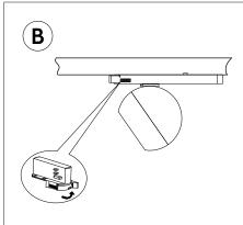
Put the adapter into the track and hook it. Choose L1/L2/L3 on the knob according to your circuit.
