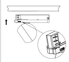
The arrow must be aligned with the "0"/"OFF" point on the knob to keep 4 pins inside.
