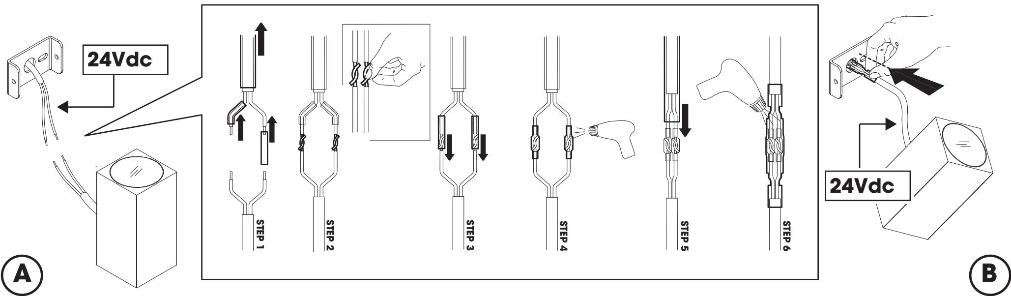
**FISSAGGIO A PARETE - INSTALLATION ON WALL**
