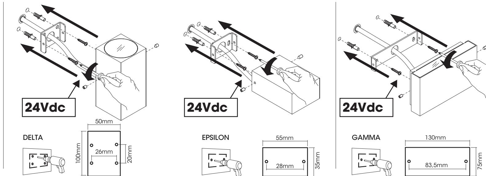
**CABLAGGIO 24Vdc - WIRING 24Vdc**
